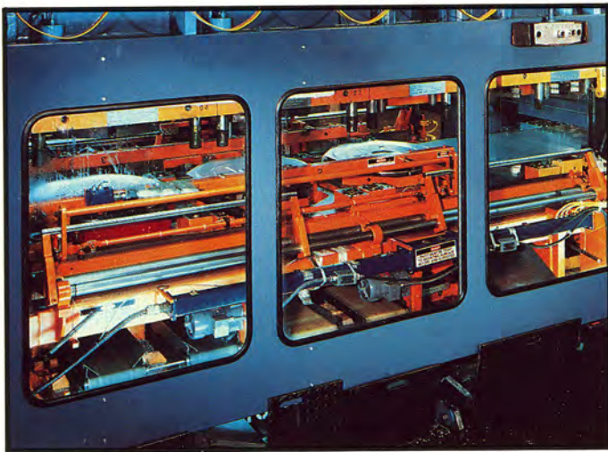
This 28" diameter drum back for a WCI dryer is produced in four stations. Previously production would have required five people and four presses.
