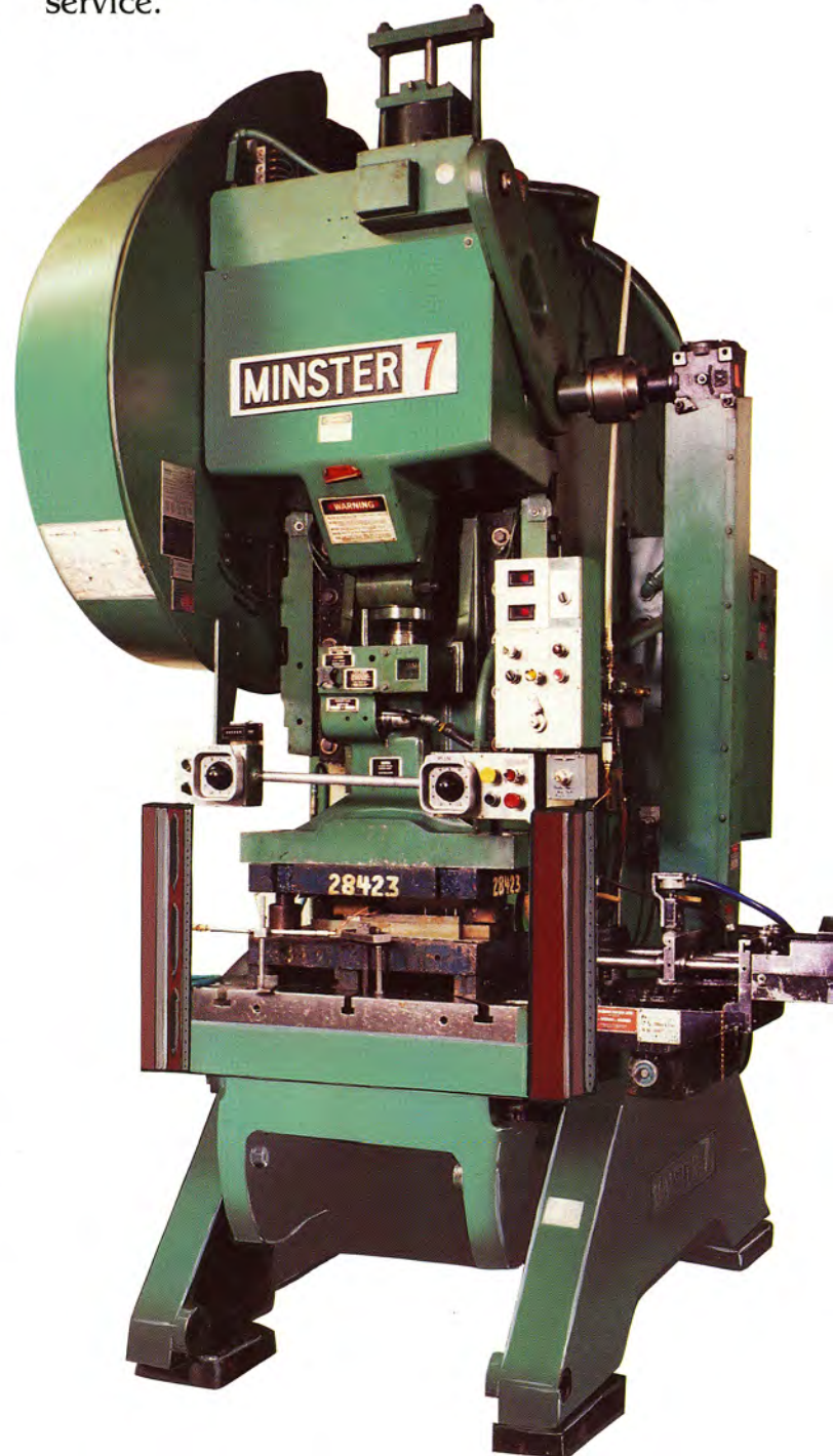
Minster 75-ton capacity O.B.I. press in production at International Tooling & Stamping, Inc., Mt. Juliet, TN.
