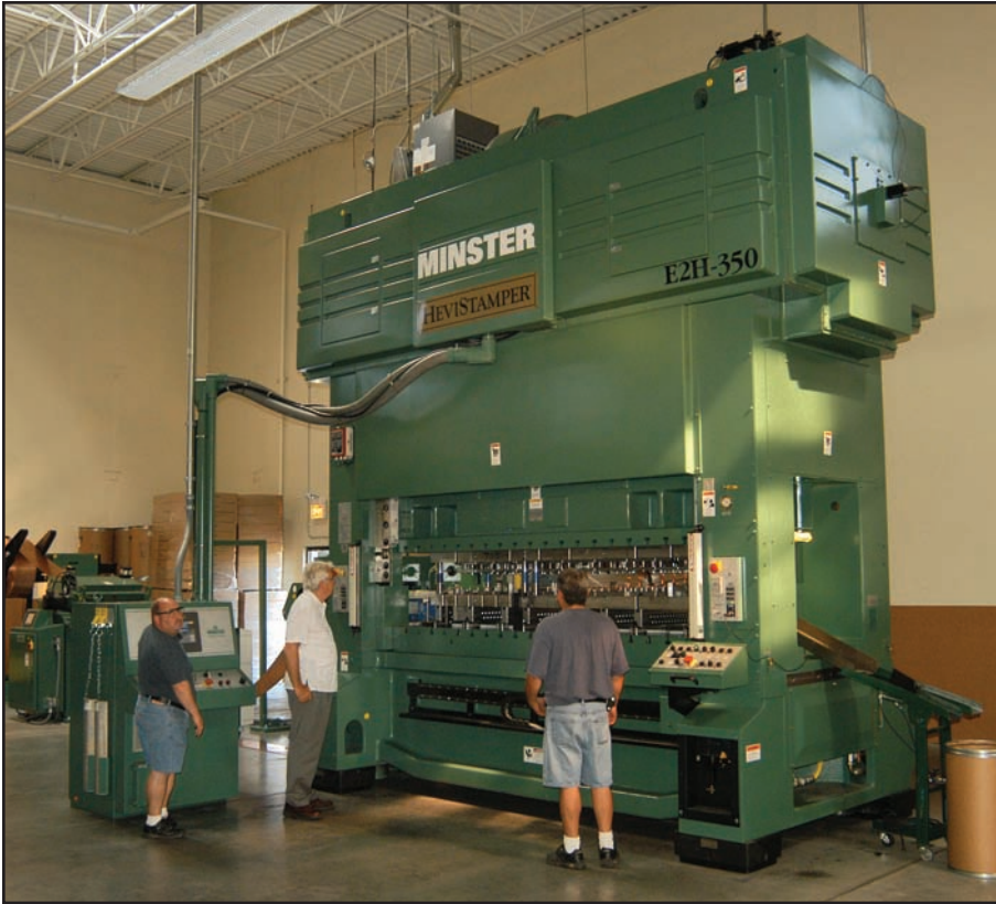
A Minster E2H-350 press with the Infinitely Adjustable Stroke option has increased the manufacturing flexibility at the Royal Die and Stamping Co.
