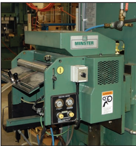
P2 press includes a Minster MEF2-CS Feed.
