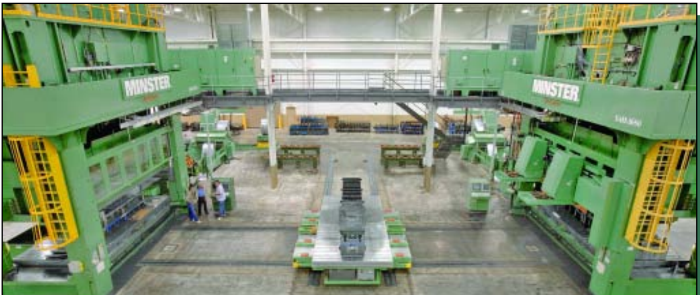
A large motorized die cart between two Minster E4H 1650 presses assists in tool changes at Wico Metal Products.
